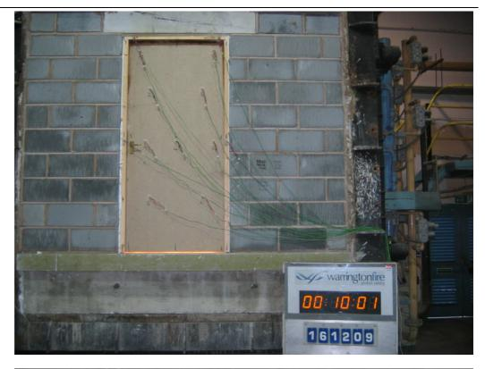
The unexposed face of the doorset after 20 minutes of testing
