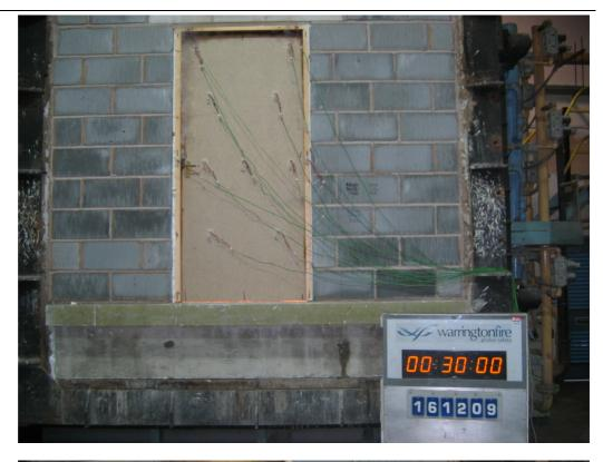
The unexposed face of the doorset after 40 minutes of testing
