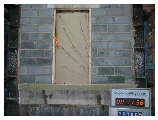
The exposed face of the doorset immediately after the test
