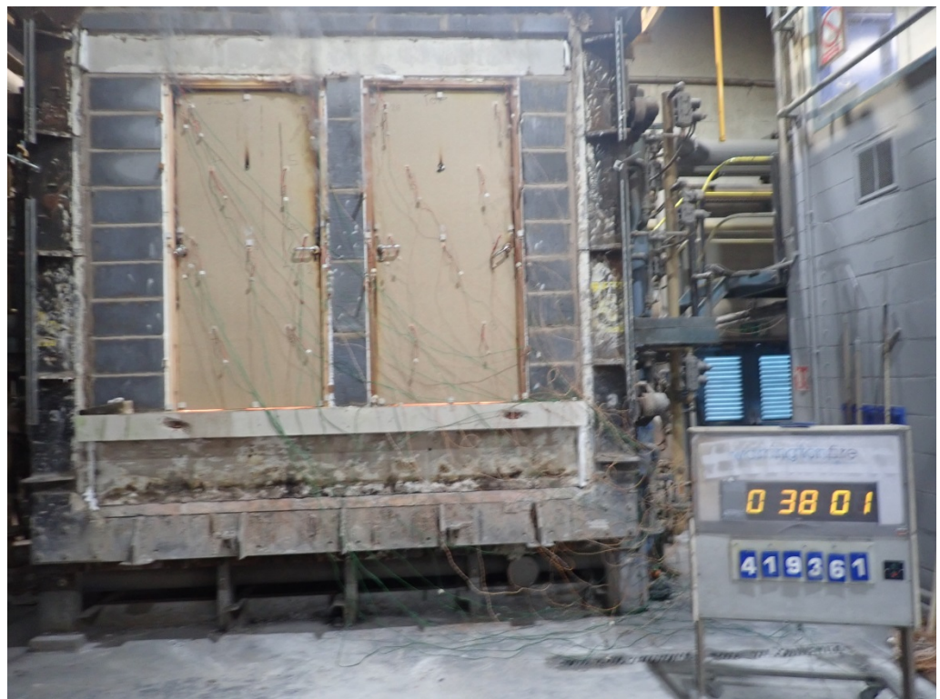
The unexposed face of the doorsets after a test duration of 38 minutes
